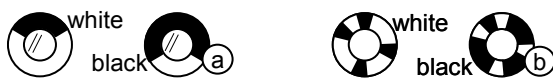
Figure 20: (a) The Markers of the checkers game (b) By adding redundancy we can make markers immune against translation.
