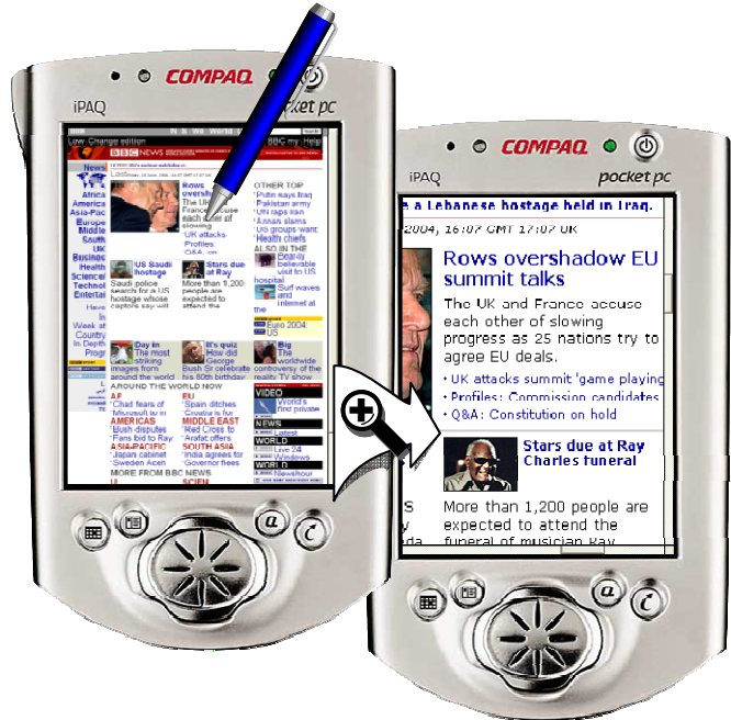
Figure 3: The zooming interaction provided by Summary Thumbnails is a semantic zoom: zooming in replaces the abbreviated text with complete text.
